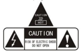
The lightning symbol points out a dangerous voltage inside of the device to hurt persons through electric shock.
