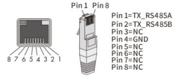
2. Unscrew the communication port cover cap in the following arrow sequence and insert the network cable into the RS485 communication client attached.
