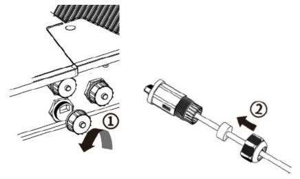
3. Insert the network cable into the corresponding communication terminal of the inverter according to the arrow sequence, tighten the thread sleeve, and then tighten the forcing nut at the tail.
