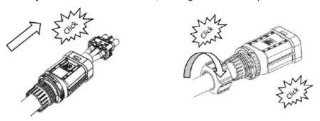
5. Insert the AC connector plug into the output socket of AC connector corresponding to the inverter and tighten them.
