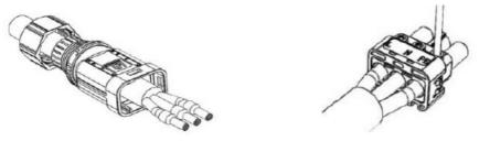
4. Secure the connector body assemble to the connector, then tighten the nut cap to the connector body.
