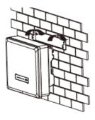
Insert wall plugs into the wall and fix the wall mounting bracket to the wall by screwing three self-tapping screws(SW10).
