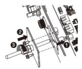
4. If a communication cover is used, remove only one sealing plug of the cable gland to thread the cable. The detailed installation process follows the above steps.
