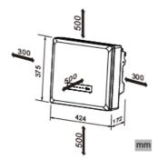
8. To ensure adequate heat dissipation, the clearances between the inverter and other objects are recommended as follows.
