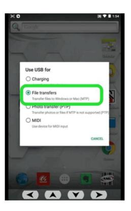
Open Windows File Explorer on the PC. (\*note: this can also be performed using a thumb drive inserted into the charging cradle) Copy your apk file(s) to: Scepter > Internal storage > Download.
