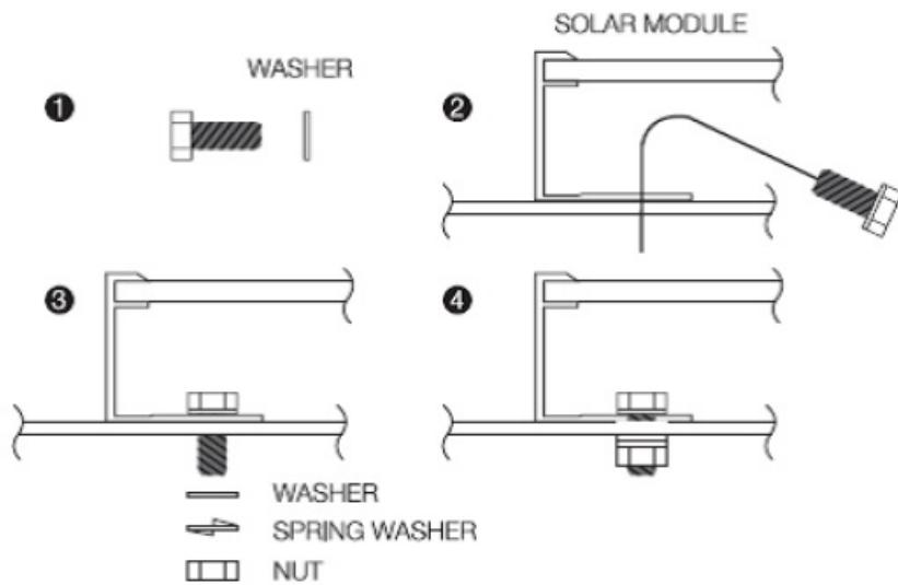
Mounting with bolts can be done only through dedicated predrilled holes in the frame. Drilling new holes is forbidden and will void the warranty.
