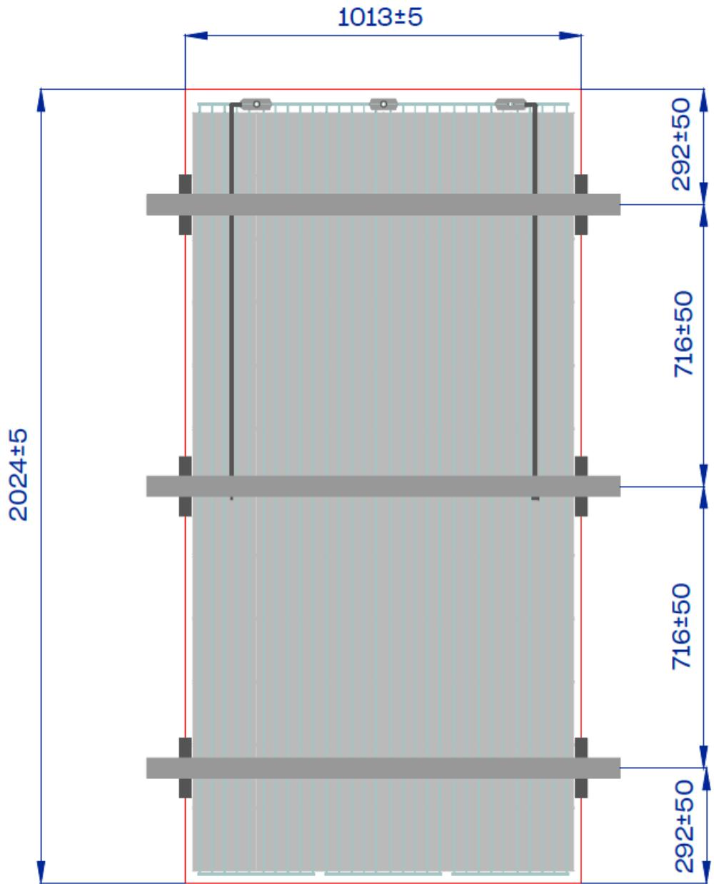
Using six Alumero CLICK 6.8 200 mm clamps allows for the panel to achieve 3600 Pa of snow loads and 1600 Pa of wind loads. It is normal that at loadings higher than 1600 Pa panels will touch the transversal rails. Please make sure that the rail surface is smooth because even the smallest sharp edge can cause fast mechanical failure. If the rail surface is not smooth, sharp edges occur, it is recommended to use rail gaskets to even the touching surface.
