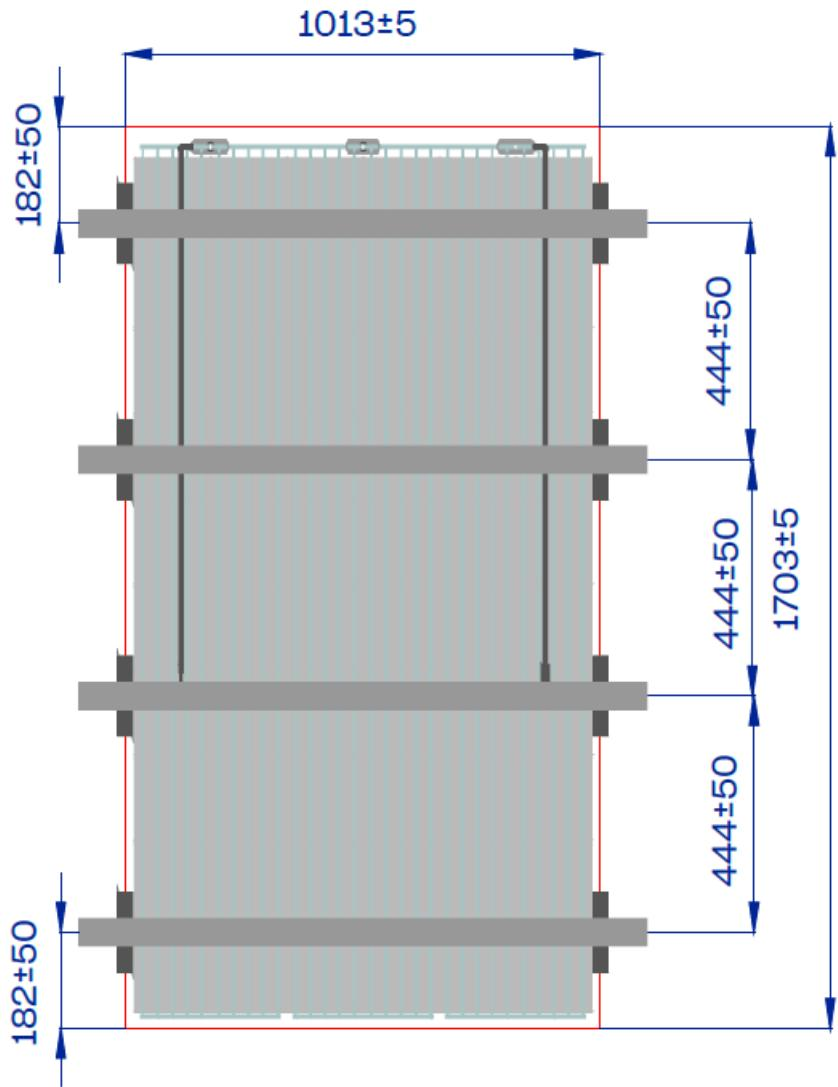
Using four Alumero CLICK 6.8 200 mm clamps allows for the panel to achieve 5330 Pa of snow loads and 1600 Pa of wind loads. It is normal that at loadings higher than 1600 Pa panels will touch the transversal rails. Please make sure that the rail surface is smooth because even the smallest sharp edge can cause fast mechanical failure. If the rail surface is not smooth, sharp edges occur, it is recommended to use rail gaskets to even the touching surface.
