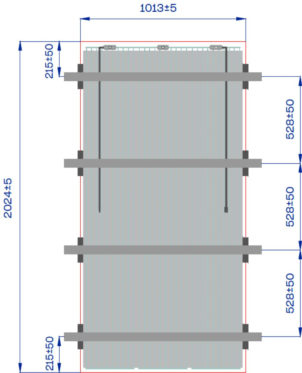
Using eight Alumero CLICK 6.8 200 mm clamps allows for the panel to achieve 5330 Pa of snow loads and 1600 Pa of wind loads. It is normal that at loadings higher than 1600 Pa panels will touch the transversal rails. Please make sure that the rail surface is smooth because even the smallest sharp edge can cause fast mechanical failure. If the rail surface is not smooth, sharp edges occur, it is recommended to use rail gaskets to even the touching surface.
