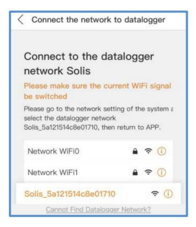
Step 7: The wireless device(mobile phone or laptop) connects to the datalogger hotspot(Solis\_serial number). The default password is 123456789.
