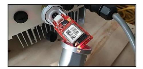
**STEP 4:** The circuitry has a small SMD button at the bottom of the antenna as shown.
