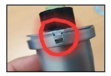
STEP 3: Now connect the upper part of the dongle back to the inverter as shown. (Important Step)
