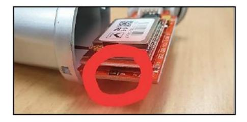
**STEP 5:** Press the SMD button for 45 x seconds. The light will switch OFF and back ON.
