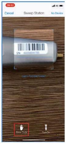
Note: Please scan the SN number of the datalogger, not the SN number on the inverter.
