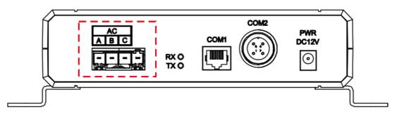
4. Connect RS485 communication cable to COM1(RJ45) or COM2(4 core connector).
