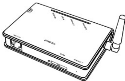
① 1 PV data logger (GPRS Box GL-G01)
