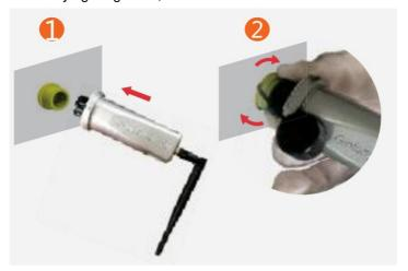
**NOTE:** The device must be installed away from the strong magnetic field produced by large electrical appliances such as microwave oven, refrigerator, telephone, metal walls.etc. Otherwise, the communication quality may be
