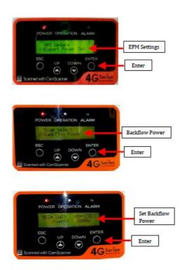
STEP 6: Use Up/Down key to scroll to EPM settings/ Internal EPM/ Export Power Set, whichever is available on your screen. Then press Enter.
