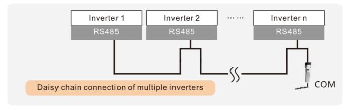
After the datalogger is installed on the inverter, if the inverter is powered on, you need to set the inverter slave address, the default slave address of the inverter is 01, and each inverter on the communication circuit needs to be assigned with different slave address(like 01,02,03,04...).
