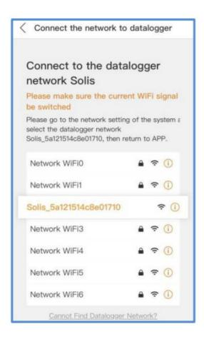
**Step 7:** The wireless device(mobile phone or laptop) connects to the datalogger hotspot (**Solis\_serial number**). The Password is 123456789.
