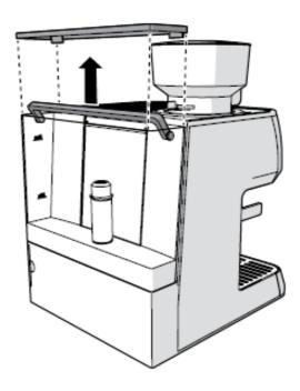
To replace the water filter cartridge:
