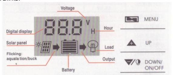
**MENU:** Switch between different display or to enter/exjt setting by long press. Up :press to increase value. DOWN:Press to decrease value.
