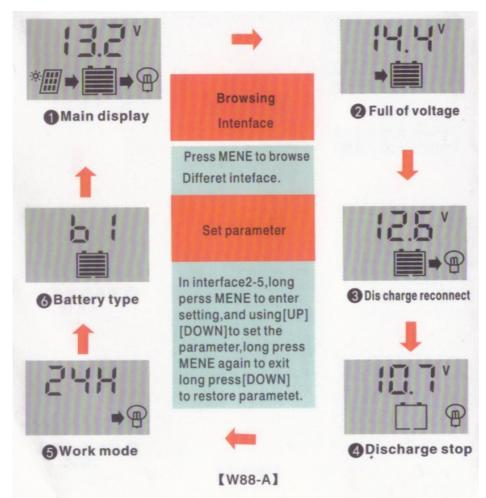
Attn: 1 .Press the [DOWN] button to ON/OF load manfully at main display. 2.The work mode is working as below. [24H] load output 24 hours [1-23H] load on after sunset and dosed after setting hours [OH] Dusk to dawn
