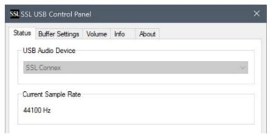
The ASIO buffer size can be adjusted from the Buffer Settings tab. This tab also shows the input and output latencies.
