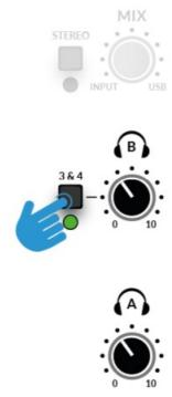
By default, the Headphones B Output with 3&4 engaged will not respect the MIX control e.g. Only DAW Outputs 3-4 are sent to Headphones B. Pressing and holding 3&4 until the LED starts to flash will allow Headphones B to respect the MIX control, allowing the artist to benefit from a mix of the low-latency input signals (Inputs 1-2), together with a custom headphone mix (3&4). You can toggle between the two modes whenever you like.
