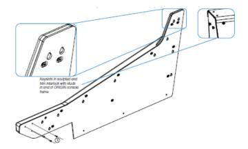
Removing the end trim starts with removing the three cross headed screws that secure the front buffer/ armrest (1 in the diagram above) and the three 2mm hex headed retaining screws (2 in the diagram on the right) on the bottom edge of the trim. With these six screws removed the trim can be gently slid up vertically to align the keyhole slots with the locating lugs and then removing the trim horizontally.
