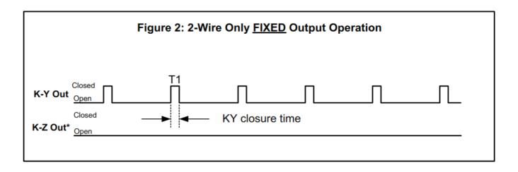
\*If the output is configured for Form A pulses the K-Z output is is not used. In Figure 2 above, the K-Z output is disabled, thus showing no pulses.
