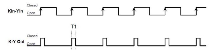
As a general guideline, the input pulse rate should not be greater than two times the output time selected. For example, if a 500mS output time is selected, the input pulse rate should be no faster than 1 pulse per second. Contact the factory for technical support at (888)272-9336.
