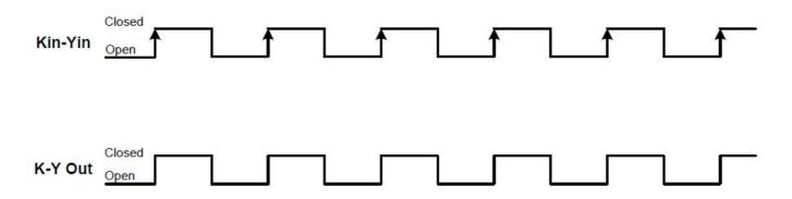
If the Fixed Mode is desired on either or both channels, set Dip Switch S1.3 UP for the Fixed mode on Channel 1. Set Dip Switch S1.6 UP for the Fixed mode on Channel 2. In the Fixed output mode, shown in Figure 2 below, an output pulse (K-Y closure) with a selected width (T1) occurs each time the input is triggered.
