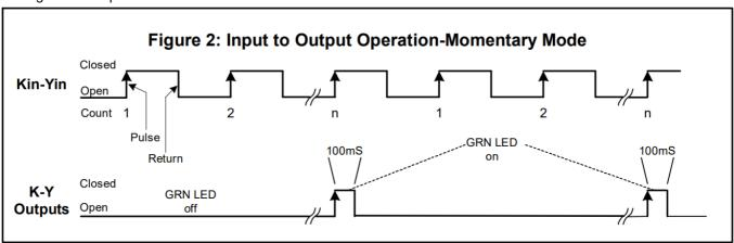
The DPR-4 can output a fixed maximum rate of 5 pulses per second of 100mS in duration, with 100mS spaces between the pulses. In the event that the frequency of incoming pulsesis high and the divider number is low, such that the output frequency exceeds 5 pulses per second, the DPR-4 will store up to 255 pulses and output them when possible. If this problem persists, a higher divider number is recommended which will result in fewer pulses of greater value.
