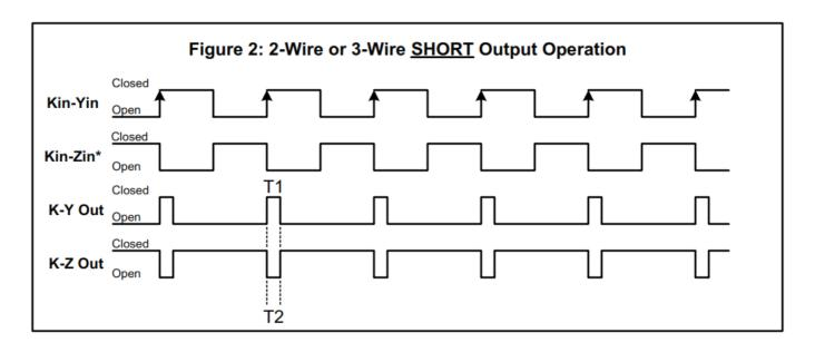
If the input pulse rate is greater than 9 pulses per second or if pulses of 100mS are too short for the receiving equipment, it is recommend that the LONG pulse output mode be used. Contact the factory for technical support at (888)272-9336.
