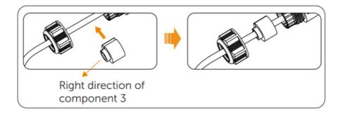
Step 3: Clockwise tighten all the components in sequence to complete the LAN assembly.
