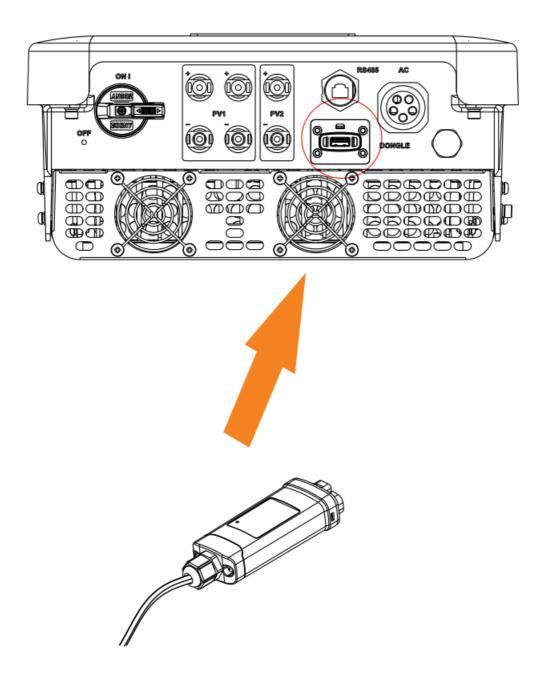
• Plug the Pocket LAN into the correct port of inverter.
