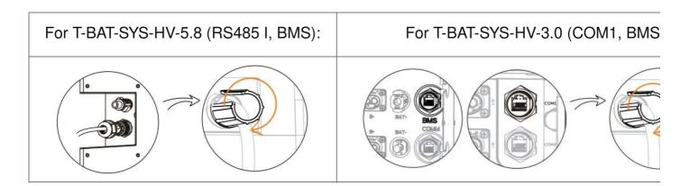
1. There is a protection cover for the RS485 connector. Unscrew the cover and plug one end of the RS485 I communication cable to the RS485 I connector. Tighten the plastic screw nut which is set on the cable with a rotation wrench. The operation is the same
