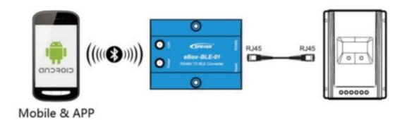
**NOTE:** Standard network cable(Parallel cable) can achieve the connection!
