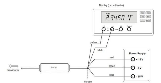
It is usual to connect cable screen to power supply 0V.
