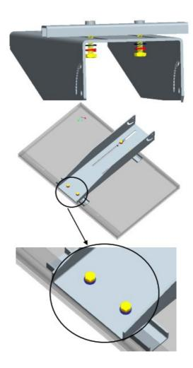
Step 2 – attaching the bracket to the pole
