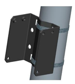
Step 3 – attaching the panel/arm assembly to the bracket Insert the bolt and flat washer from the inside out
