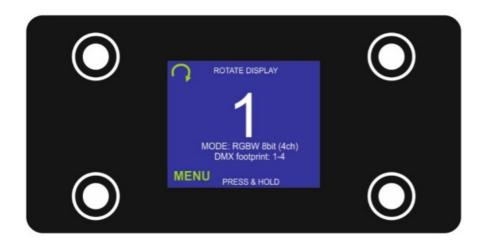
Press and hold the **<MENU>** button to scroll through the top-level menu items. Use the and buttons, located to the right of the LCD screen, to navigate the menu map and menu options. Press the  $< \checkmark >$  button to access the menu function currently displayed or to enable a menu option. To return to the top of the menu map or menu without changing the value, press the < X > button.
