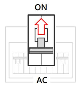
2. Turn on the inverter ON/OFF/P switch and DC safety switch (if applicable).
