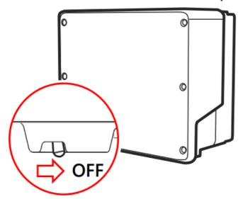
2. Turn off AC to the inverter on the main service panel.
