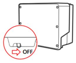
2. Turn off AC to the inverter on the main service panel.
