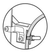
4. Mount the inverter cover and Connection Unit cover (if applicable). Tighten the screws to 8.4N·m/74lb-in.
