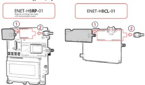
3. Tie the antenna cable to the communication board bracket with a plastic tie (supplied).
