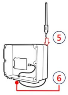
6. Pass the antenna cable through a communication gland.
