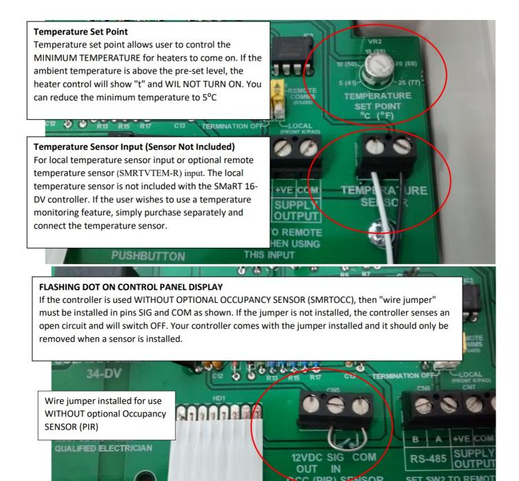
**PLEASE NOTE:** If you are using a SMRTOCC with the Solaira SMaRT 16DV and 34DV, the timer function on the SMaRT Wall Switch SM-WSD will be overridden if the SMRTOCC has been activated. If you are not using a SMRTOCC, the Link that is fitted as standard between the SIG IN / COM 'MUST' be removed otherwise the timer function on the SMaRT Wall Switch SM-WSD will not operate.
