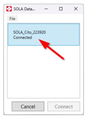
Once connected, a message will be displayed in the message area indicating that a device with a specific name is connected. Disconnection is done either by connecting to another device in the list, or by turning off the device. When a device is disconnected, a message is displayed in the message area.
