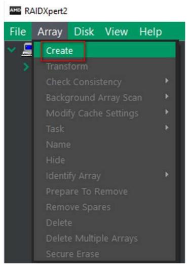
8. Select the RAID type, the disks which would like to use for RAID, volume capacity and then create the RAID array.
