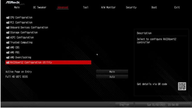
7. Go to Advanced\RAIDXpert2 Configuration Utility\Array Management, and then delete the existing disk arrays before creating a new array.
