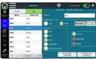
Important: Before running a test, it is necessary to select the correct type of cable, otherwise the result could be affected.
