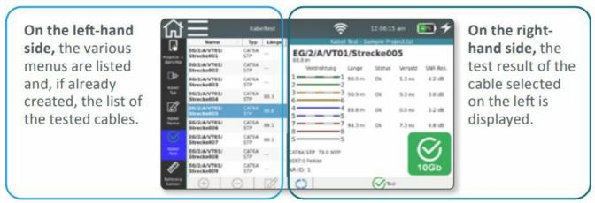
A qualification test can directly be started by tapping the Test button.
