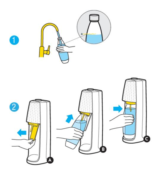
**Note:** when inserted correctly, there is a small gap between the bottom of the Carbonating Bottle and the base. Do not carbonate if the Carbonating Bottle is resting on the base, or water will splash out.
