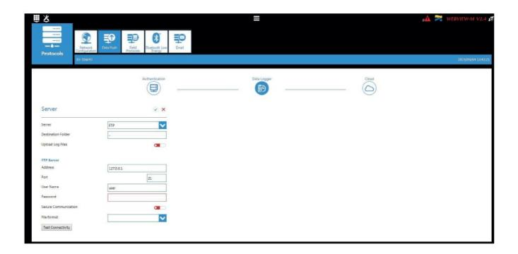
Server: activate the FTP server to enable the automatic export of data to a remote FTP server.
