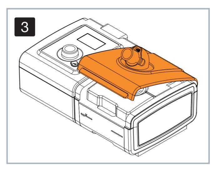
4. Guide the adapter hose down into your reservoir through the port making sure that the hose on the underside passes into the reservoir opening and rests near the bottom. Attach the adapter to your reservoir.
