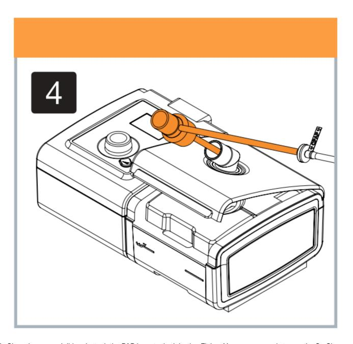
5. Close the reservoir lid and attach the PAP hose to the Injection Fitting. You are now ready to use the So Clean.
