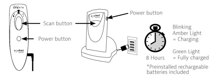
Charging Requirements: Min 5.0 VDC, 1 AMP Max 5.5 VDC, 3 AMPs
