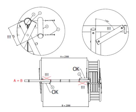
**NOTE**For the safety of your children, the accessories should be installed according to the drawings below!
