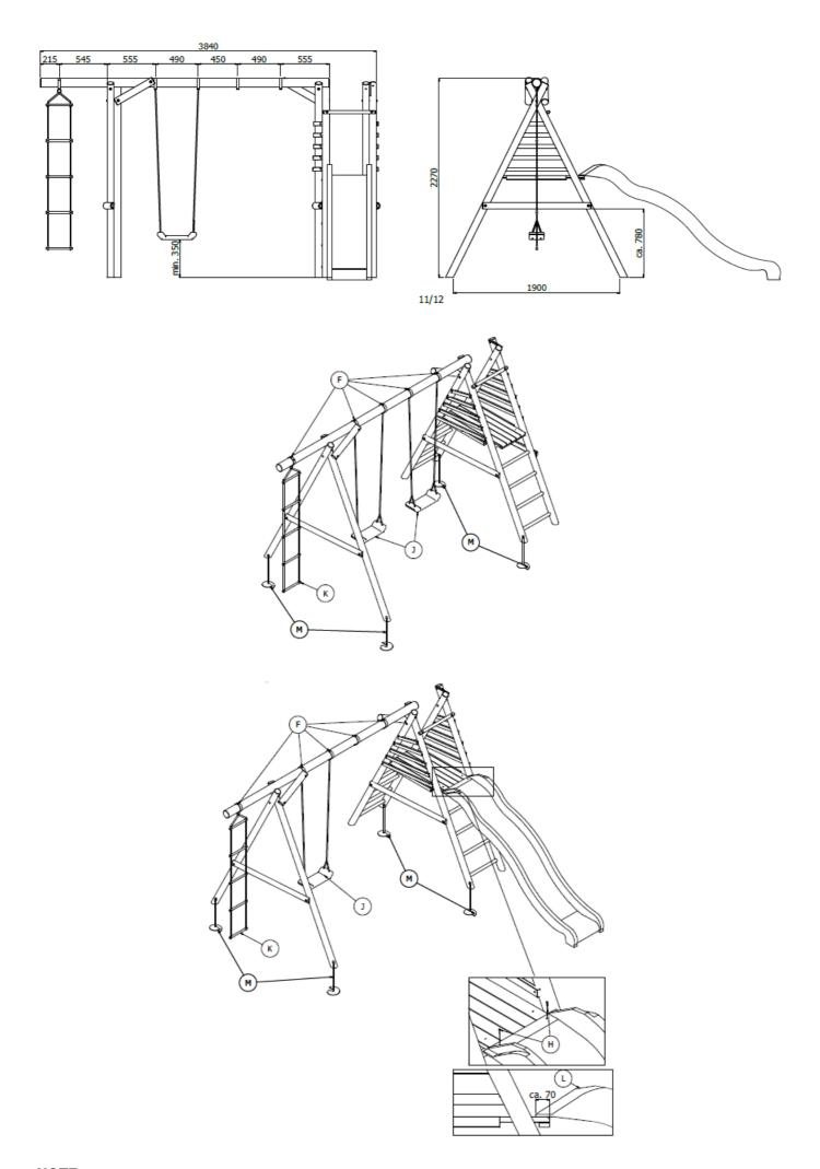
Ground anchors (K) which should be used in order to attach the swing set to the ground. The anchors are not included in the kit, they have to be purchased separately. Installing the anchors is necessary to ensure the stability of the swing set and to minimize the risk of its tipping over.
