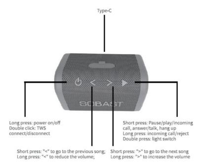
Bluetooth connection: After the speaker is turned on, it enters the Bluetooth pairing state. Search for the Bluetooth name "S21" on the mobile phone and click to connect. Connect.
