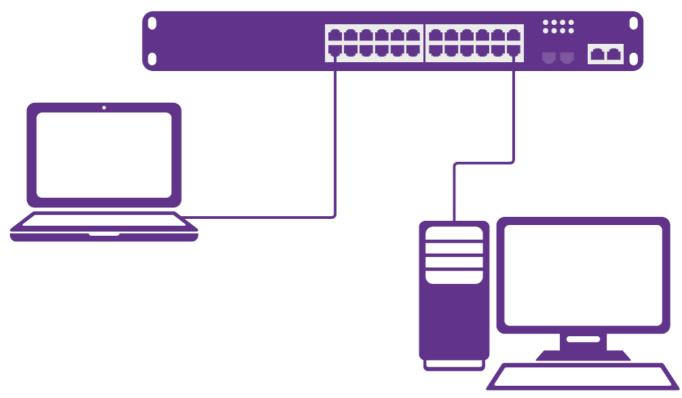
Connect the Switch with the PC NIC interface. Power on the Switch. Check whether the IP-address of the computer is within this network segment: 192.168.1.xxx ("xxx" ranges 2~254), for example, 192.168.1.100. Open the browser, and enter http://192.168.1.1 and then press «Enter» or open telnet connection to address 192.168.1.1.
