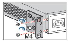
Fix the captive nuts and install the device in a cabinet. Attention: leave more than 1U space between the devices for proper heat dissipation.
