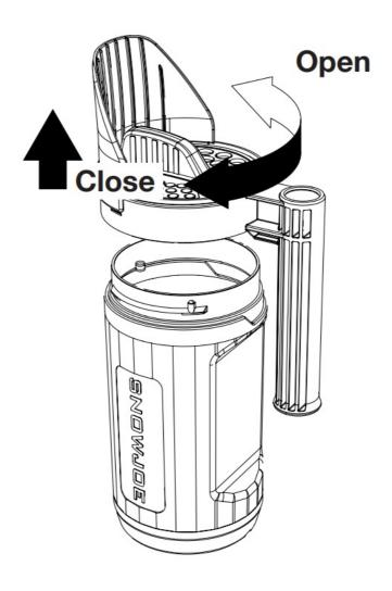
Twist the cap counterclockwise to open the spreader and fill as needed. Replace the cap and twist clockwise to secure after refilling.
