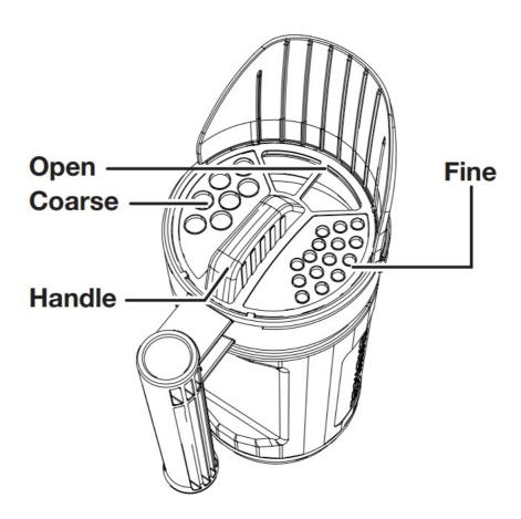
Grab the handle and twist to choose from the 3 openings based on the specific need. This allows you to control the flow rate of various sizes of ice melt, seeds, fertilizer, pool chemicals, and more.
