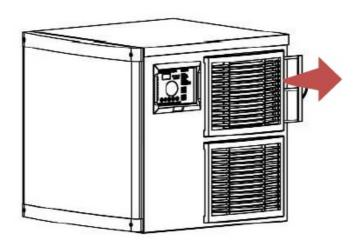
Note: Be careful when doing the condenser cleaning as the edges of the fins are sharp.
