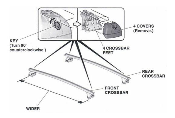
Check the identification marks, and position the front and rear crossbars on the roof rails.
