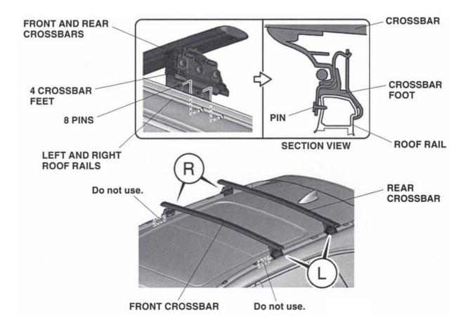
To line up the crossbar pins with the roof rails, you may need to slightly loosen the crossbar screws. Make sure each clamp is fully seated on the roof rail as shown. Loosely tighten each screw, then torque them to 3.0 lb-ft (4 N-m).
