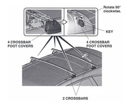
Make sure the crossbars are firmly secured by applying pressure to them as shown. Store the keys and special tool in a safe place.
