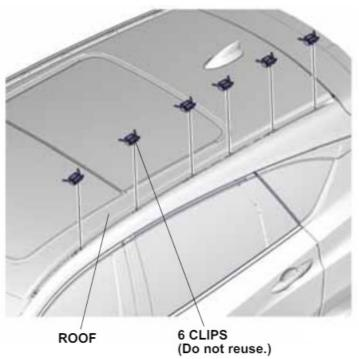
3. Install the left roof rail to the roof with six TORX nuts.
