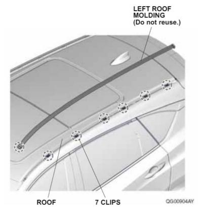
2. Remove the six clips from each stud bolt on the roof.
