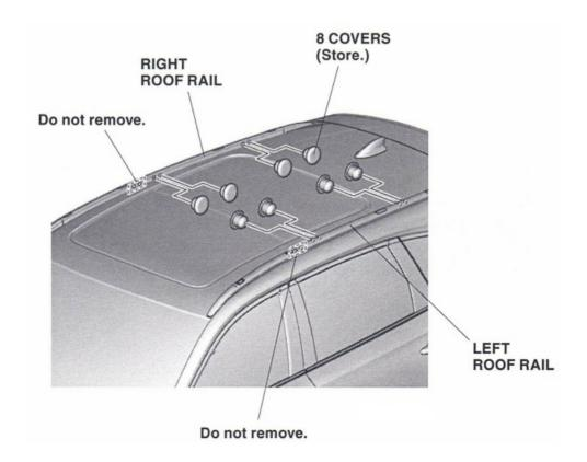
On each crossbar toot, turn the supplied key 90° counterclockwise to unlock the cover. Then, remove them. Identify the front and rear crossbars as shown.
