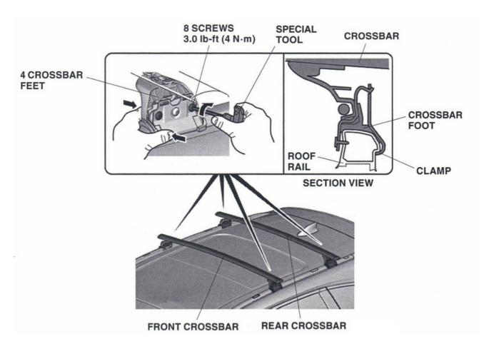
Install the crossbar foot cover to the crossbar foot with firm pressure. Then, rotate the key 90° clockwise, and remove it. Repeat for each crossbar foot.
