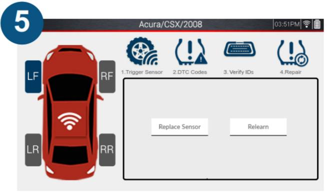
Continuing on to Repair, selecting either Replace or Relearn will take you to that screen at the main TPMS function where you can program a sensoror perform a relearn
