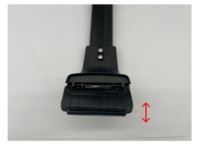
4. Using the provided wrench, loosen the bottom bolts on the four clamps.
