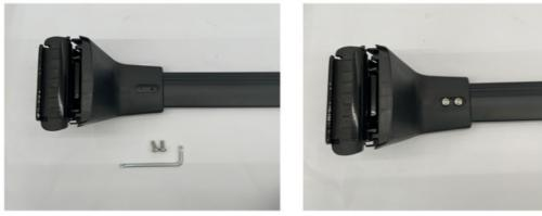
2. Install the screws by the supplied wrench. Tighten each screw but allow the crossbar to be able to slide in the mount. The screw will be tightened once it is mounted on the car roof.
