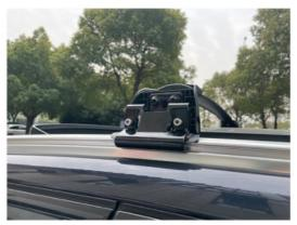
6. Mount the correct bar on the suitable location. Make sure the rubber piece is not pinched and is flat again the rail, which will protect the roof rail.
