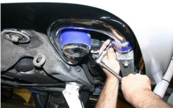
Install upper IC inlet pipe into the two silicone couplers along with 2.56" t-bolts on each side. Position the Tbolts as shown and tighten down all the way if everything is aligned correctly. If not, reposition as needed then, tighten clamps. Now go back and finish tightening the bottom IC inlet clamps that you left loose. (see above)
