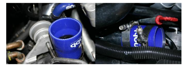
Install the 2.25" straight coupler to the top of the lower IC inlet pipe with a supplied 2.56" Tbolt, tighten all the way. (Above right)
