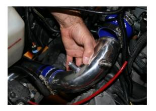
Position the 90 degree throttle body pipe into the Throttle body coupler and into the 2.5" coupler from the lower FMIC outlet pipe. Position it so that is it snug up against the lower coolant pipe then tighten all the clamps on the outlet side. (Remember to tighten the IC outlet clamps that you didn't tighten earlier) (below left.. next page)
