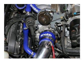
Next install the Lower Idle air control motor hose to the FMIC piping. The motor may need to be rotated slightly or the IC pipe may need to be moved closer to the throttle body for this to fit on. Tighten with the small (included) worm clamps. (above right)
