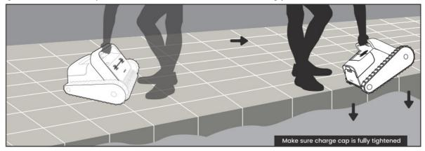
Hold it in water for a few seconds as it releases air trapped in it.
