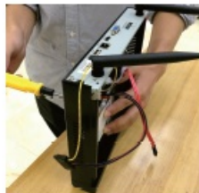
Insert the hard drive, secure it to the bottom of the unit with the four screws
