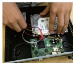
Connect the data wire and power wire as shown
